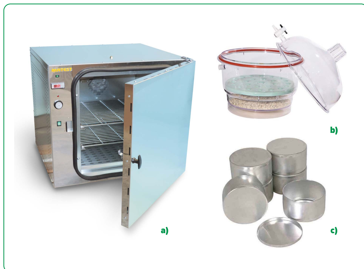
Figure 48. a) oven, b) desiccator; and c) metal dishes, for measuring moisture content using the oven-drying method ( matest.com ; coleparmer.co.uk ; certifiedmtp.com ).
