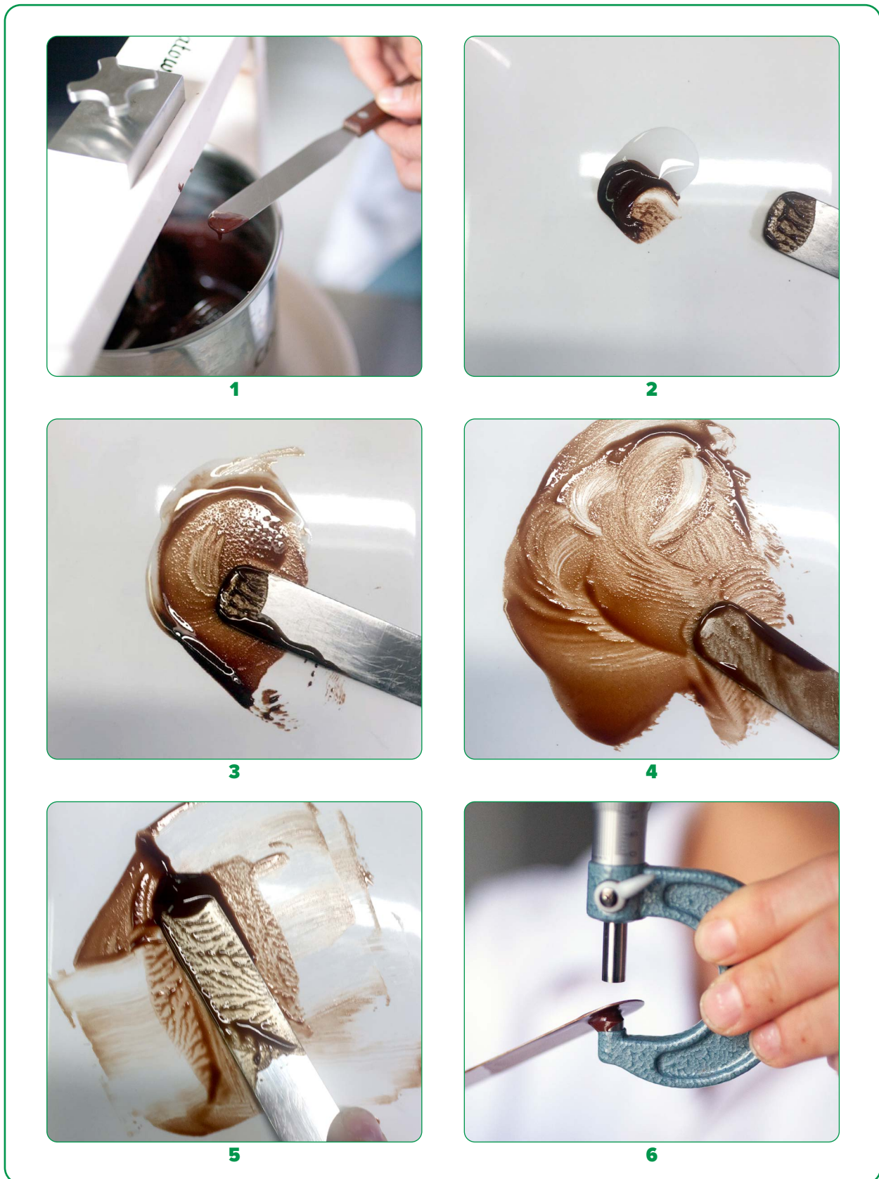
Figure 38. Cacao mass preparation procedure using mineral oil, for measuring particle size with a micrometer (Bioversity International, Archila, 2022).
