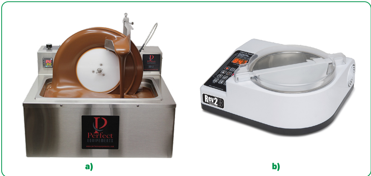
Figure 82. Semi automatic tempering machines: a) rotating wheel tempering machine; b) rotating bowl tempering machine. ( perfectchoco.com ; chocovision.com ).
