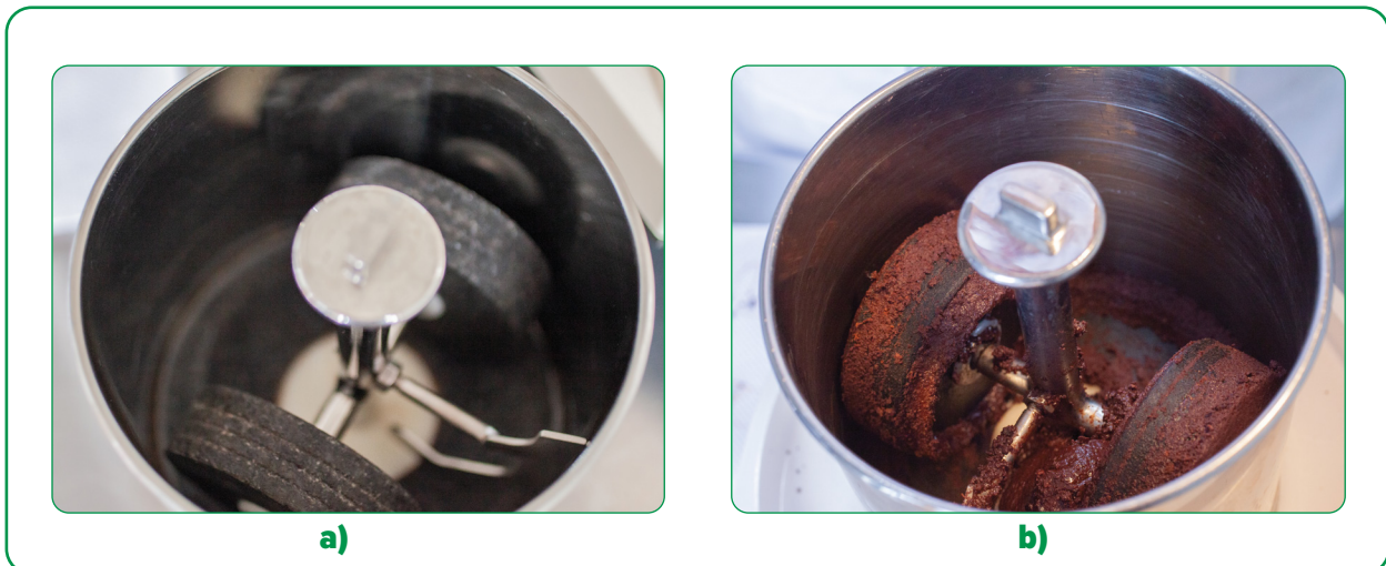
Figure70. Inside the melanger: a) view of stone grinder assembly inside the empty stone bowl; b) view of the melanger bowl while grinding cacao nibs into cacao mass. ( chocolatemelangeur.com ; chocolatealchemy.com ).
