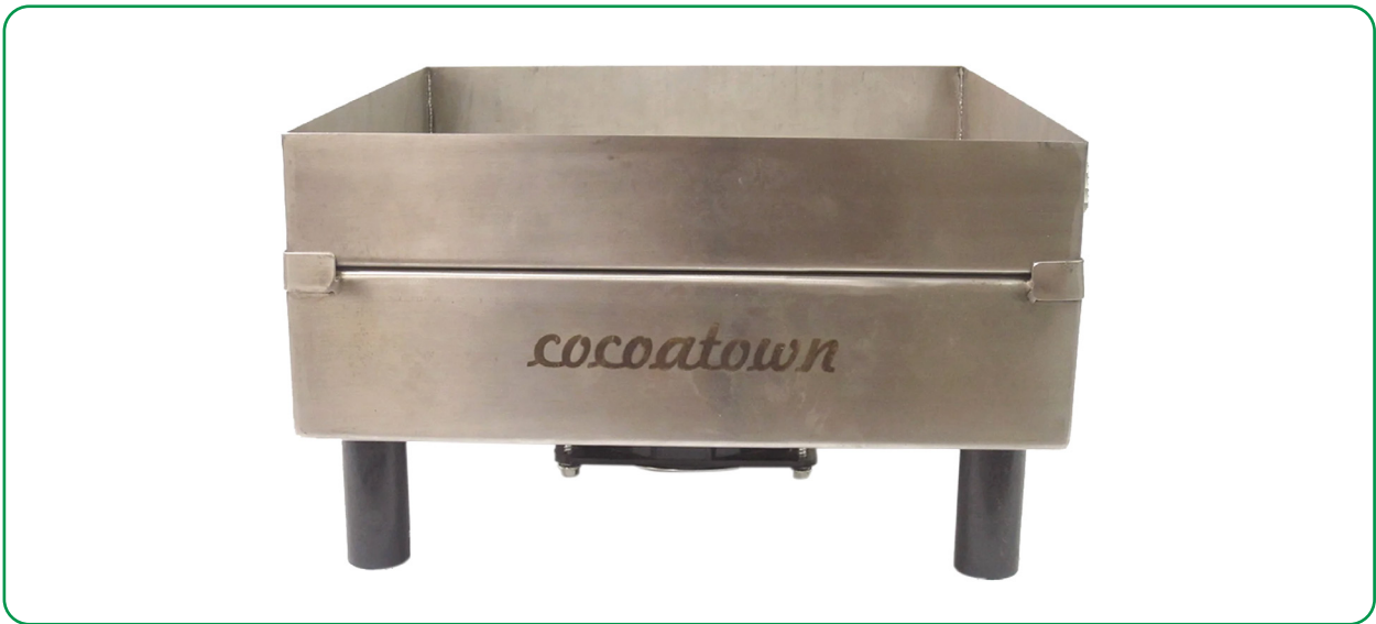
Figure 61. Example of cooling tray with fan attached at the bottom ( cocoatown.com ).
