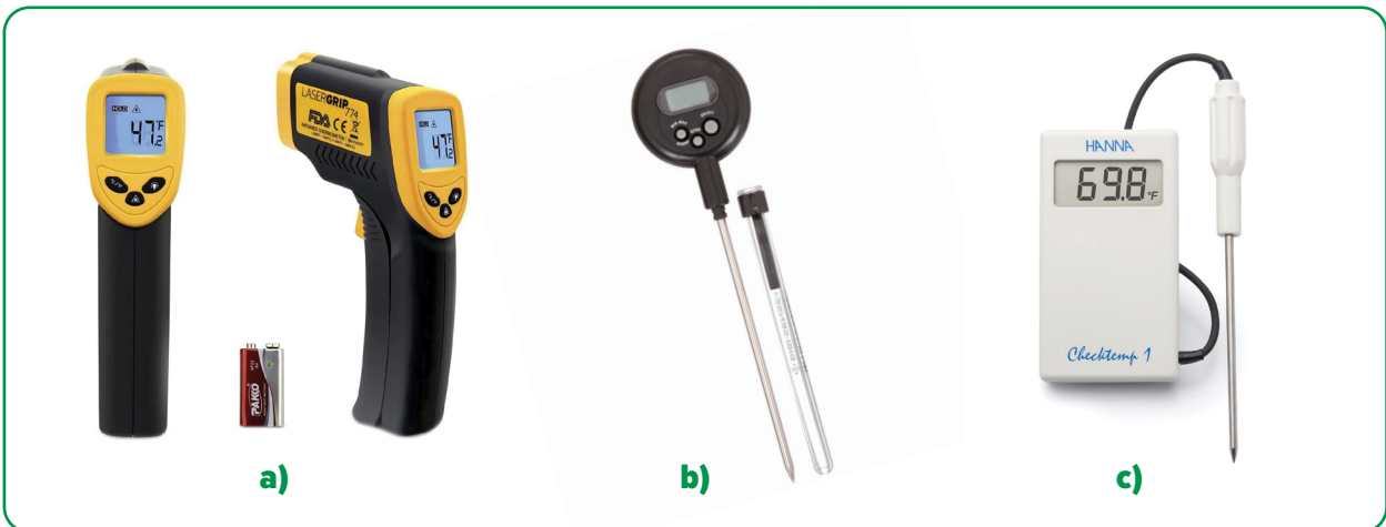
Figure 79. Examples of digital thermometers: a) infrared thermometer; b) stem thermometer; c) probe thermometer ( etekcity.com ; coleparmer.co.uk ; hannainst.com ).
