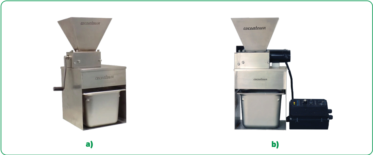
Figure 65. CocoaTown™ cacao bean crackers a) Manual Cracker; and b) Power Cracker ( cocoatown.com ).
